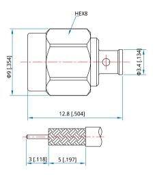
Unit: mm [in] Tolerance: ±0.2mm [±0.008in] Connector
